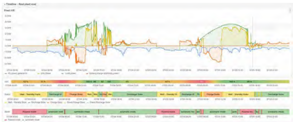
Figure 32 Dashboard example visualizing 2 reference days of MPC applied to the real system. The first chart reports the time-series of applied load (blue), PV production (green), operation of battery (red) and resulting metered net
