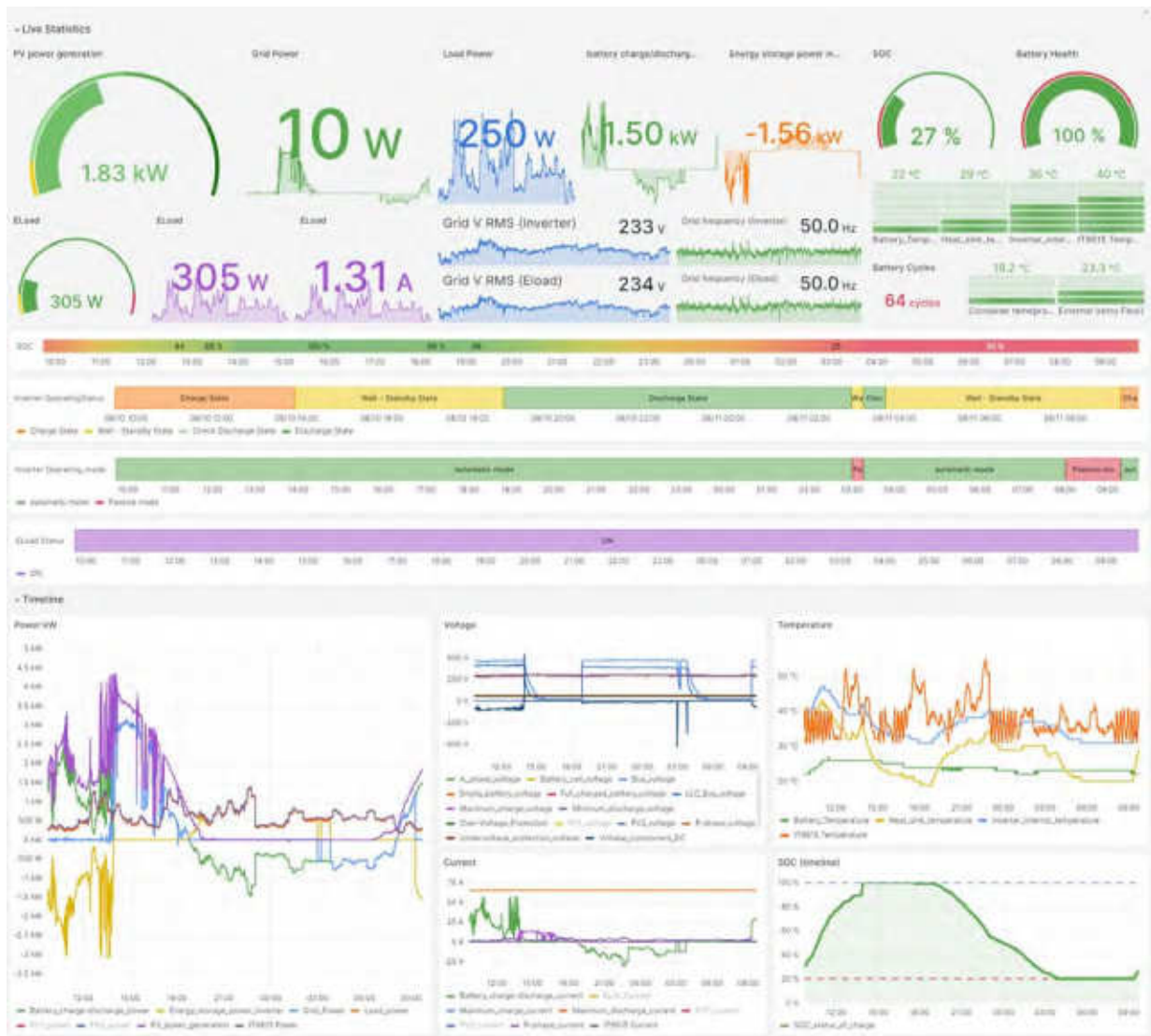
Figure 29 Grafana 19 dashboard to monitor the operation of the experimental plant. Live data and past 24h overview of main collected measures (image taken the day 2023-08-11).
