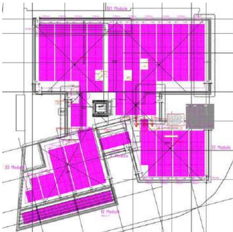
FIGURE 16 - INSTALLATION OF THE 190 PV-PANELS ON THE ROOF TYPE AC-410MH/108V. 12 SEMI-TRANSPARENT MODULES WITH 210 Wp/MODULE.
